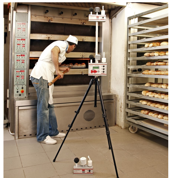
Three levels WBGT on the same vertical
