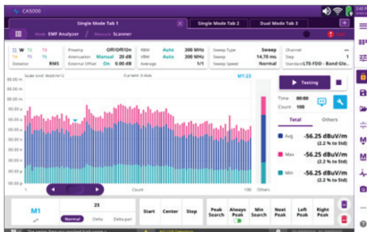
OneAdvisor 800 Wireless EMF Scanner (frequency selective mode)
