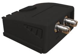
Allows to measure the differential pressure  $\Delta P$  and to calculate air velocity and airflow with a **Pitot tube** or **Debimo blades**. It also measures the thermocouple temperature with a wired thermocouple probe ended with a male miniature connector.
