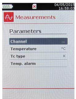
For all probes and modules, it is possible to modify the channel number.
