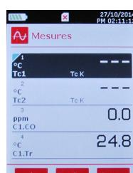
In "Measurement" menu, press the function key "Channels".
