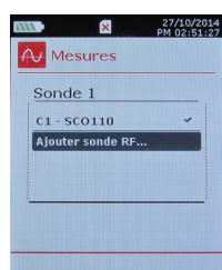
With the arrow keys, select "Add wireless probe..." then press OK.
