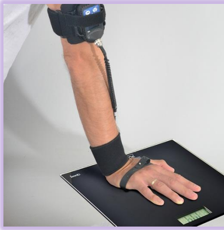
Figure 4-7 Using a bathroom scale as reference level for the contact force check
