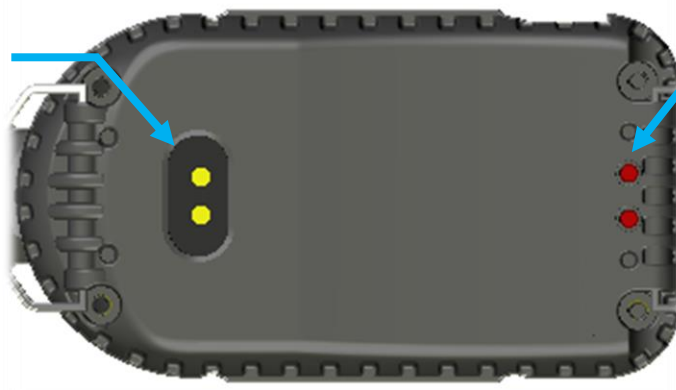
Figure 3-3 SV 103 back view - charging and infrared port (reserved for future use)
