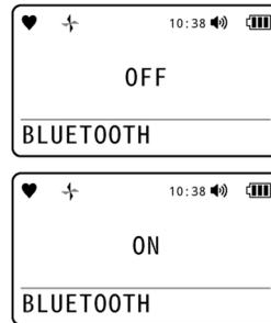
The Bluetooth device connection is set. [SETTING] appears followed by [END], and the display returns to the screen in Step 1.
