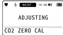
Once CO<sub>2</sub> zero adjustment has been successfully completed, the result is displayed, and the concentration after CO<sub>2</sub> zero adjustment is then displayed.
