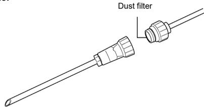
**3 Rotate the probe to attach it.**
