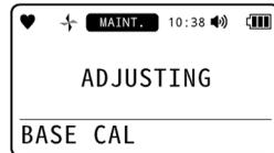
Once base gas adjustment has been successfully completed, the result is displayed, and the concentration after base gas adjustment is then displayed.
