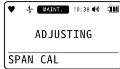
Once span adjustment has been successfully completed, the result is displayed, and the concentration after span adjustment is then displayed.
