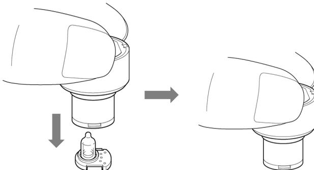
**<Installing the VOC sensor>**
