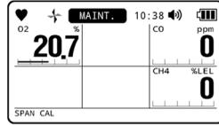
Span adjustment is performed.
