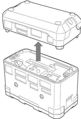
\* The diagram shows the lithium ion battery unit.
