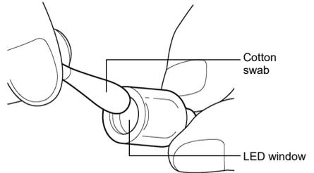
**3 Use a clean cotton swab to remove any remaining alumina polishing powder from the LED window.**
