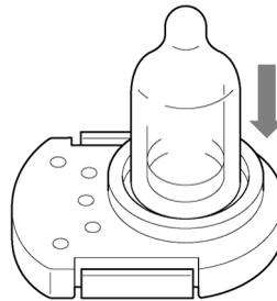
**4 Place the pellet into which the LED has been fitted on a flat surface. Place the VOC sensor main unit over it and press so that the pellet fits into the VOC sensor main unit.**
