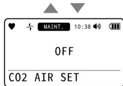
3 Press the POWER/ENTER button. Whether to perform fresh air adjustment for the carbon dioxide sensor is set. [END] appears, and the display returns to the screen in Step 1.
