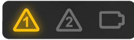
Flashing amber warning 'icon 1' will be illuminated when the STEL threshold is exceeded.
