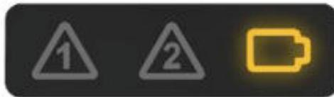
The battery icon will flash amber intermittently (three seconds) to indicate a power status between 69 and 40%.
