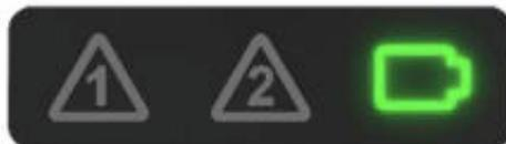
The XD One heartbeat is indicated via the intermittent flashing (three seconds) of the battery icon.
