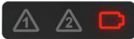
The battery icon will flash red intermittently (three seconds) to indicate a power status of 39% or lower.
