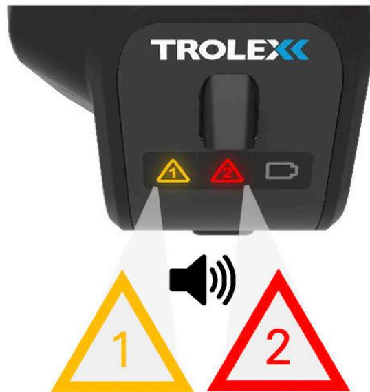
If a threshold is breached during operation, the following alarm sequence is used to alert users.
