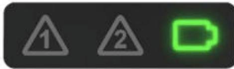
The battery icon will flash green intermittently (three seconds) to indicate a power status between 100 and 70%.
