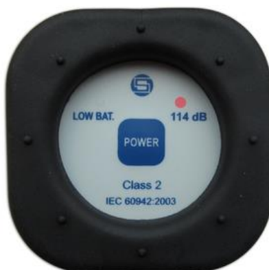
Figure 3. The top view of the SV 34B calibrator with the 114 dB LED lit
